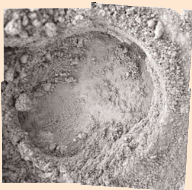
Figure 2. An 8.9-mm-deep hole cut into a rock by Opportunity .
