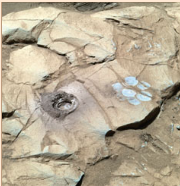
Figure 1. Spirit's rock abrasion tool drilled a hole (left) and brushed the surface (right) off a rock nicknamed "Clovis".
